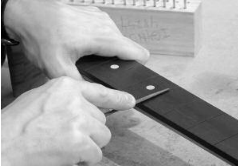
13.70: Using a small triangular file to break the edges of the fret slots.
