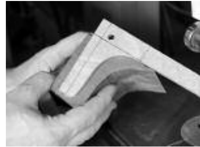
13.23: The neck shaft side template is used to layout the rough shape of the heel block. Use the full size diagram supplied when you make your side template.
