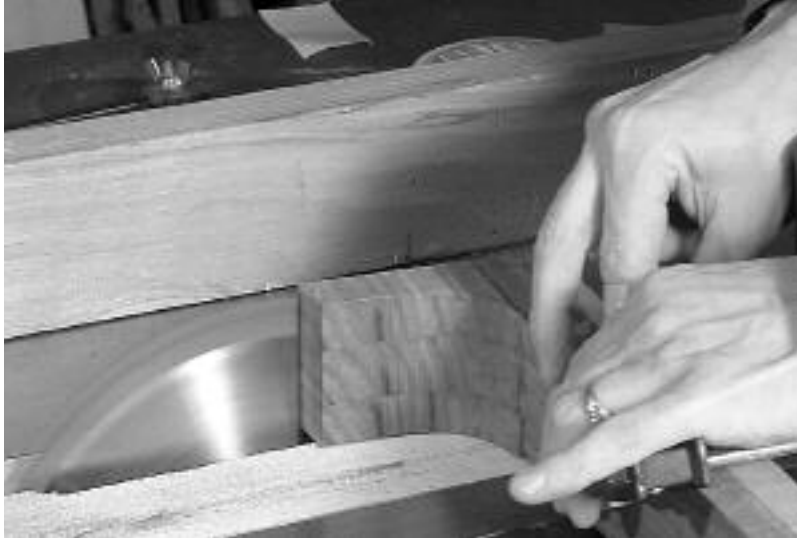
13.54: Cutting the heel angle with the neck securely clamped to the miter gauge.
