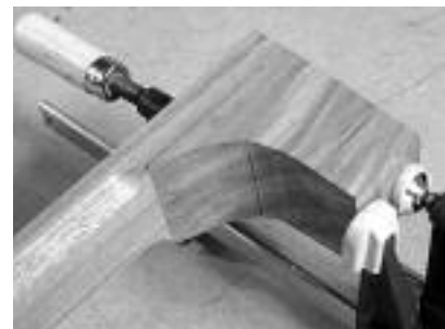
13.26: Clamp the block to the neck shaft just behind where the neck shaft chamfering ends.
